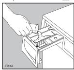
If required, pour fabric softener into the compartment marked **8** (the amount used must not exceed the "MAX" mark in the drawer). Close the drawer gently.
